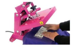
Align the transfer material on the garment to be printed.
