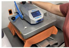
3 This will be a COLD peel, so be sure to move the garment off the heat press and over to the side to cool off.
