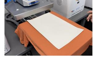
2 For the final press, use the glossy side toward the transfer and press for 5-8 seconds with medium to heavy pressure at 360° F.
