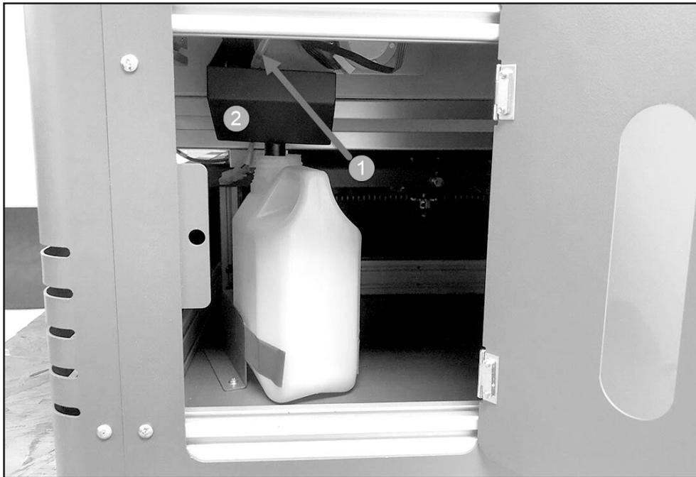
3. Remove Female Luer Fitting from Waste Tube and Replace with Blue Male Luer Fitting and M2 Check Valve and Insert Waste Tube Back into Waste Funnel
