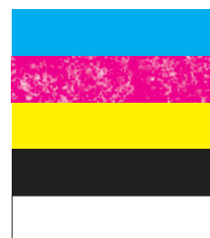
Printing with a WORN Magenta image drum
