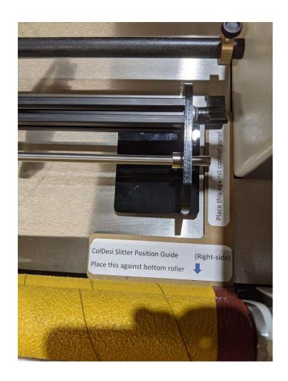
\*\*PLACEMENT OF THE CARDBOARD CUT-OUTS IS SOLELY DEPENDENT ON THE LENGTH OF THE VERTICAL BLADE ASSEMBLY, DRY FIT THE ASSEMBLY BEFORE PEELING OFF TAPE LINERS.
