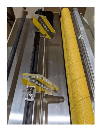
BLADES CAN BE SAFELY TUCKED INSIDE THE BLADE-HOLDERS WHEN NOT IN USE. EACH BLADE HOLDER HAS ITS OWN KNURLED SCREW.
